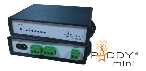
power the relay module and briefly press the «prog» button. One LED lits up to indicate programming mode.
